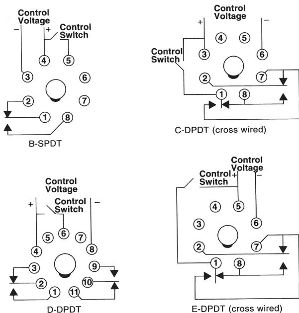
The **Duplexor** is used in control panels where **two loads** are required to alternate to provide equal run time on the loads. The alternating action is initiated by a control switch, which is common with one side of the control voltage. The output contacts will change states each time the control switch is opened, thus alternating the two loads. The LED indicators show the position of the output relay.
