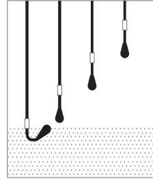
As the fluid level rises, the OFF switch closes, no loads are energized.
