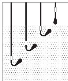
When the fluid level falls and each float switch opens, the loads remain energized so long as the OFF switch remains closed. No external auxiliary contacts are required to accomplish this latch feature.
