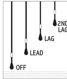
This example illustrates the normal operation of the Triplex Controller in a pump down application with four normally open dry float switches. The switches are designated off, lead, lag, and 2nd lag. The example begins with all switches open and all loads de-energized.
