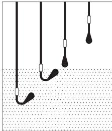
When the lag switch opens, load 1 de-energizes. Loads 2 and 3 remain energized.
