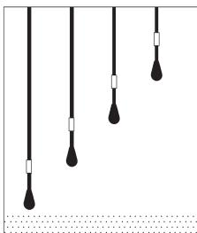
When the OFF switch opens, load 3 de-energizes and the lead advances three positions. At the end of each cycle the lead advances one position for each load energized during the cycle. This particular example reverts back to SOSO OPERATION 1-4 wherein load 1 would again be the lead load.
