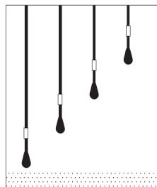
When the fluid level falls below the OFF switch, all loads simultaneously de-energize, and the alternating logic advances one position. The next rise and fall in fluid level and successive operation of load switches will result in the SOSO load operation as follows: 2-3-1, 3-1-2, and back to 1-2-3 as in Step 1.
