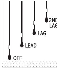
This example illustrates the normal operation of the Triplex Controller in a pump down application with four normally open dry float switches. The switches are designated off, lead, lag, and 2nd lag. The example begins with all switches open and all loads de-energized.
