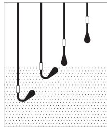
If the fluid level continues to rise, the lead switch closes and load 1 energizes.
