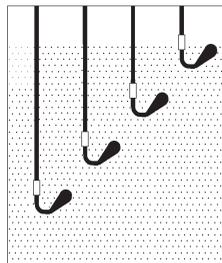
As the fluid level continues to rise each successive float switch closure sequentially energizes a corresponding load.
