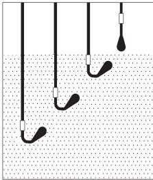
As the fluid level falls, the 2nd lag switch opens. All loads remain energized. Each float switch in descending order acts as the OFF switch for the preceding float.
