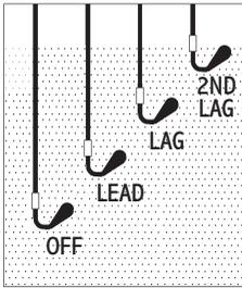
This example continues from SOSO operation step four. With all float switches closed, all loads are energized.
