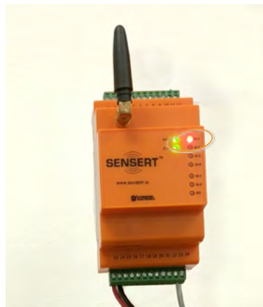
Once saved, you will see that the SENSERT unit will turn on the AI-1 (Analog Channel 1) by illuminating the LED status.
