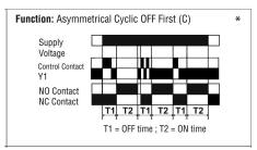
To have the load being on for T1 time followed by off for T2 time repeated until the end of the total timing duration, Function D Asymmetrical Cyclic Off First will be used. For this method you will need to jump terminal A1 to terminal 25 of the 175MD.
