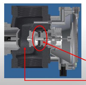
The monitor module will activate when the system experiences a failure such as the main valve disk is stuck open or the lever disengages from the valve stem assembly. When the P303 main regulator fails to regulate and the output pressure climbs, the increased output
