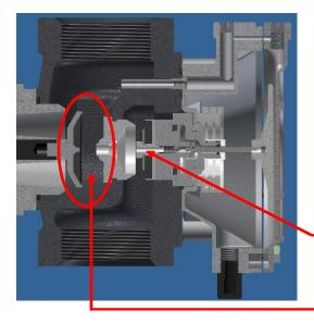
Under normal operational conditions, the P303 Series performs as the P300. When there is a demand downstream of the regulator, the main valve disk moves away from the orifice to allow flow. The Monitor diaphragm and piston are always in motion based on outlet feedback though the pitot tube at the outlet.
