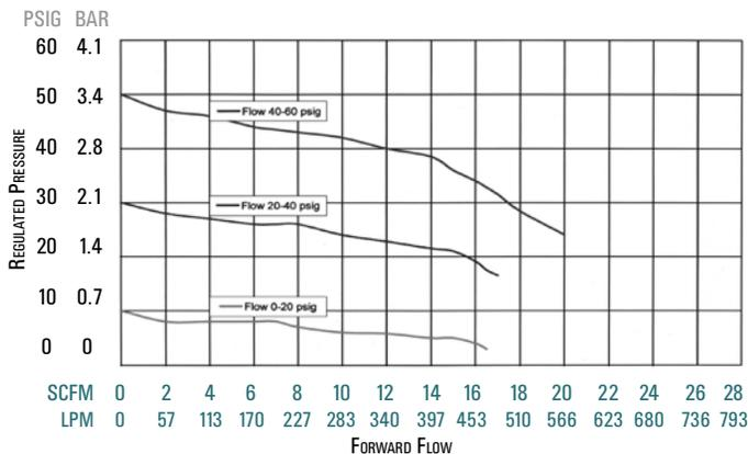
**Type 65: Regulated Pressure VS. Flow**
