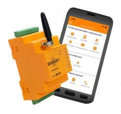
SENSERT<sup>TM</sup> is a remote process monitoring and alert system. A variety of sensors, such as temperature, humidity, vibration, and pressure, can be hardwired directly to the SENSERT Base Unit or wirelessly connected via the SENSERT Remote I/O. Sensor data is monitored in real-time and alerts are triggered based upon customizable thresholds.
