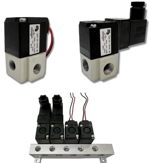
The T2200 series direct operated poppet valves are compact in size, provide large flow capacity and low power consumption. The T2200 valve is a single valve, multi ported for 2 way and 3 way operation. Options include standard and continuous operation, standalone use or manifold and flying leads or DIN terminal. The manifold mounted valve can be easily operated through PLC control in robotics and automation installations.
